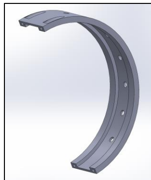
Figure 6: Two of the above lock rings bolt together to hold modules in place.
