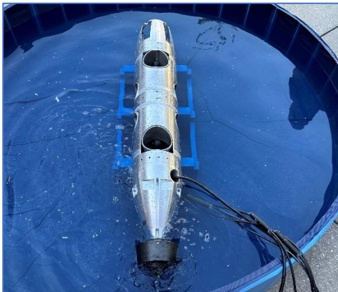
Figure 10: Subassembly used to test thrusters and how they respond to different PWM inputs.
