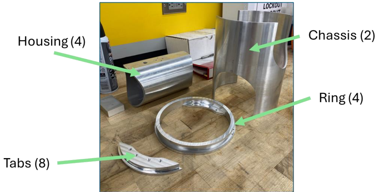
Figure 7: Individual fabricated components for thruster module.
